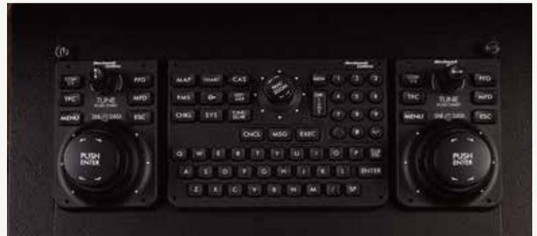
*Simple controls offer another way for you to navigate around the flight deck without using the touch screen.*
