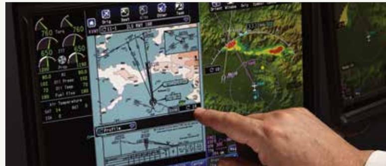
Flexible, split-screen approach charting allows quick reference to the flight path.
